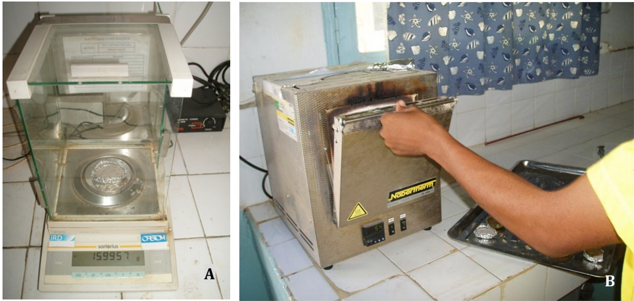
Figure 06. Analysis of sediment sample (weighting and carbonisation). A: Precision analytical balance; B: Muffle furnace.
